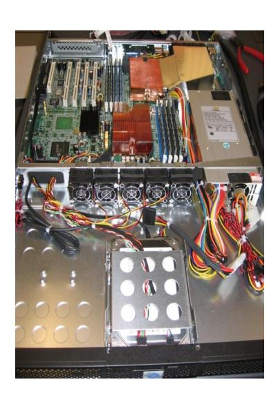
Cell G: 2 NVidia K80 GPUs, Intel E5-2640 (16-cores)
